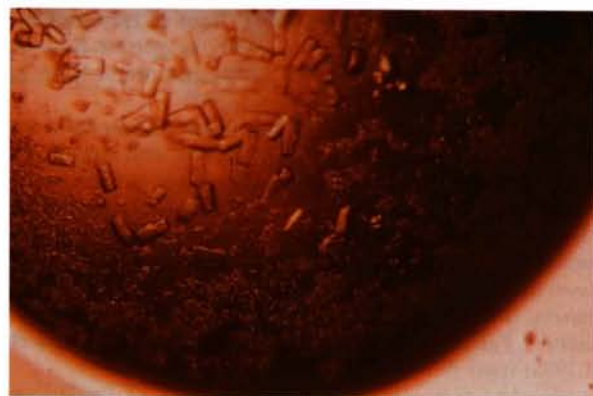
Fig. 2. Chunky plates of PeIL grown from 1,6-hexanediol and isopropanol. The longest dimension of the largest crystals is approximately 0.1 mm.
