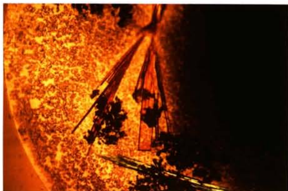
Fig. 1. Rosettes of elongated lathes of PeIL grown from PEG and isopropanol. The largest crystal (at the left) was cut free and used to collect the initial native data. After cutting it free (making the longest dimension shorter) the crystal was approximately 0.6 \times 0.1 \times 0.02 \text{ mm} with b as the long axis.
